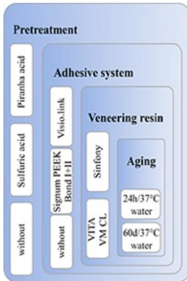
Fig. 2. Test design of TBS measurement with universal testing machine.
