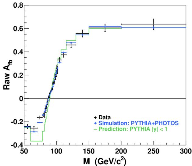
FIG. 12. Raw  $A_{\text{fb}}$  measurement in bins of the muon-pair invariant mass. Only statistical uncertainties are shown. The PYTHIA  $|y| < 1$  asymmetry curve does not include the effect of QED FSR.
