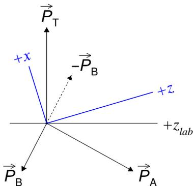
FIG. 1. Collins-Soper coordinate axes ( $x, z$ ) in the lepton-pair rest frame, along with the laboratory  $z$  axis ( $z_{lab}$ ). The three axes are in the plane formed by the proton ( $\vec{P}_A$ ) and antiproton ( $\vec{P}_B$ ) momentum vectors within the rest frame. Relative to the laboratory  $z$  axis, the transverse component of  $-(\vec{P}_A + \vec{P}_B)$  is the same as the transverse-momentum vector of the lepton pair in the laboratory ( $\vec{P}_T$ ).
