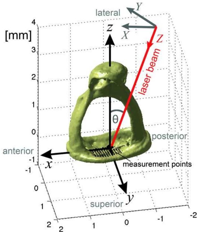
651 **Fig. 1** SLDV measurement frame ( $XYZ$  coordinate system) and footplate-fixed anatomical
