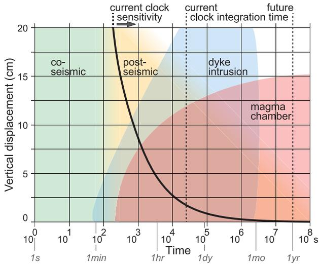
**Figure 1.** Phenomena that could be monitored with optical clock networks. The black line shows the lower sensitivity of today's best optical clocks; see eq. (1) and  $\Delta z_{\text{today}}$  in eq. (7). The vertical dashed lines show current and planned clock integration times.
