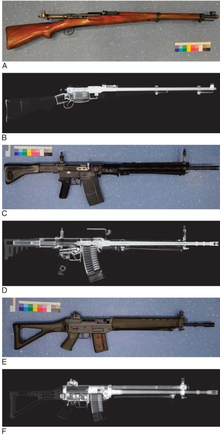
**FIGURE 2.** Rifles of the Swiss Army. A, Photography and (B) CT-reconstruction of the Karabiner 1931. C, Photography and (D) CT reconstruction of the Sturmgewehr 57. E, Photography and (F) CT reconstruction of the Sturmgewehr 90.
