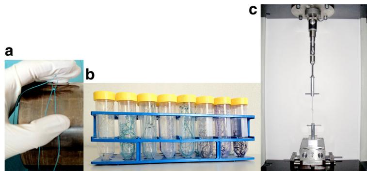
**Fig. 1** Preparation, incubation and testing of the suture loops. **a** Creating the suture loop by knotting around a metallic cylinder. **b** Six loops of the same suture material are incubated together in a polyethylene tube containing 50 ml of an approved standard testing solution. **c** Fiber loop fixed in material testing machine over a metal bar on each side
