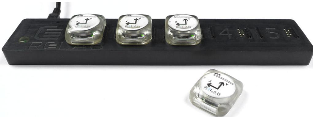
Figure 1: ReSense sensor modules and base station [24]. The base station allows data readout, battery charging and temporal synchronization of up to 5 sensor modules simultaneously via a USB 2 port.
