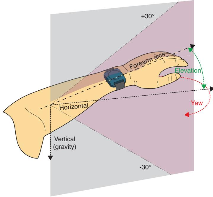
Figure 2: Illustration of the forearm angles extracted from the IMU. Elevation is the angle between the horizontal and the forearm axis and yaw is the angle covered in lateral movements. The red area in the vertical plane illustrates the region where gross arm movements are identified and movements outside of this area are not captured by the algorithm. It has to be noted that shoulder abduction, flexion and rotation as well as elbow flexion can influence elevation and yaw.
