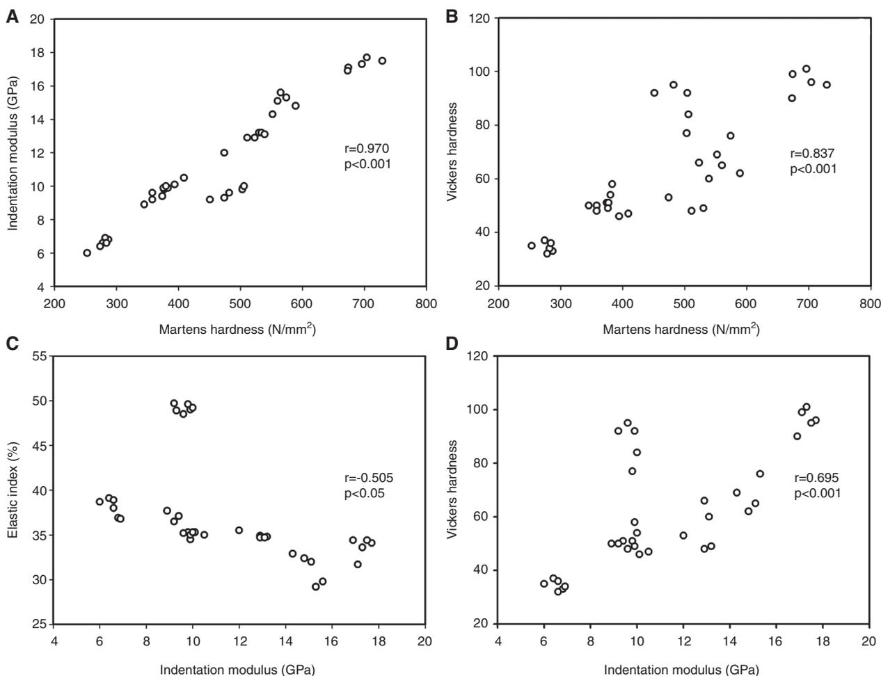
**Figure 3:** Graphical presentation of correlations between the properties tested with  $r$  and  $p$  values after Pearson analysis. (A) Martens hardness vs. indentation modulus, (B) Martens vs. Vickers hardness, (C) indentation modulus vs. elastic index and (D) indentation modulus vs. Vickers hardness.
