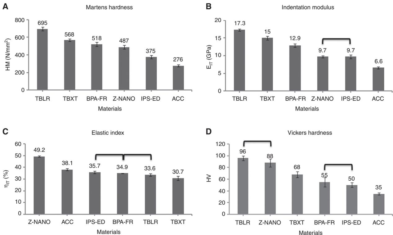
**Figure 2:** The results of the mechanical properties tested in descending order. Lines above columns connect mean values without statistical significant differences ( $p > 0.05$ ). (A) Martens hardness, (B) indentation modulus, (C) elastic index and (D) Vickers hardness.
