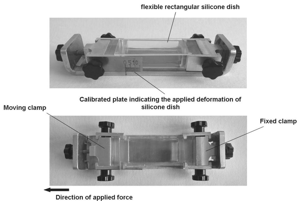
**Figure 1.** Static stretching apparatus. The rectangular flexible silicone culture dish is held at one end by a fixed clamp and the opposite end by a moving clamp. Strain magnitude can be modified manually by the knob of the moving clamp. A calibrated plate, attached to the moving clamp designating the deformation applied to the flexible silicone dish.
