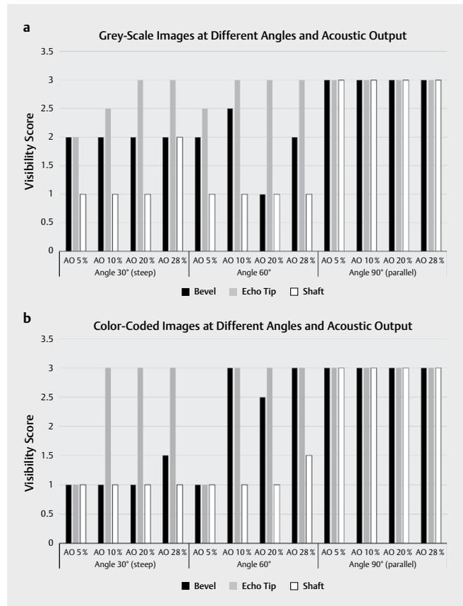
► **Fig. 6** a Comparison of different needle insertion angles and acoustic output at High Resolution preset: on grayscale **a** and color-coded **b** images increased acoustic output and angles increased needle visibility. Visibility scores: 1 = needle not visible, 2 = poorly visible, and 3 = well visible.
