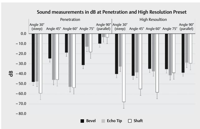
► **Fig. 5** Ultrasound measurements in needle region-of-interest show higher ultrasound reflection (recorded signal level in dB) for EchoTip® between 30° and 60° for the High Resolution preset explaining the superior visibility scores of ► **Fig. 3b** for this preset. As a reference, the level of the contrast-enhanced background tissue was between -dB 50 and -dB40. The acoustic output was 10%.
