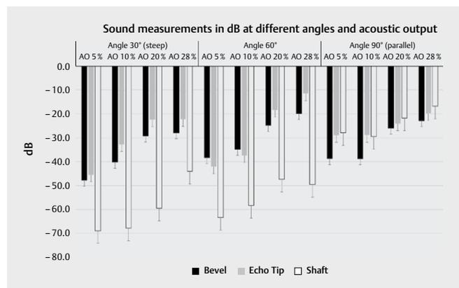
► **Fig. 7** Ultrasound measurements in needle region-of-interest show higher ultrasound reflection (recorded signal level in dB) of needle bevel, EchoTip® and shaft with increasing acoustic output (AO) and insertion angles. The highest dB values were obtained for the needle shaft parallel to the linear probe. The High Resolution preset was used.
