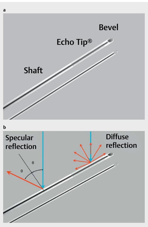
► Fig. 2 a Detail view of the 18G Chiba biopsy needle shows a) bevel, followed by EchoTip<sup>®</sup> and shaft and b) different reflection characteristics of EchoTip<sup>®</sup> and shaft. The lower needle is the internal stylet. Picture: Permission for use granted by Cook Medical, Bloomington, Indiana
