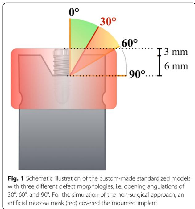
**Fig. 1** Schematic illustration of the custom-made standardized models with three different defect morphologies, i.e. opening angulations of 30°, 60°, and 90°. For the simulation of the non-surgical approach, an artificial mucosa mask (red) covered the mounted implant
