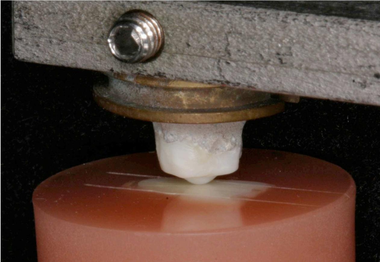
Example of the contact between enamel specimens and antagonist. Track length of linear attrition amounted to 3 mm. For better visibility, the adhesive tape covering the identification marks and limiting the test surface for erosion to 1.5 mm width was removed.
