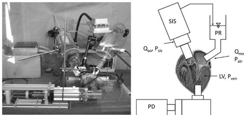
**Figure 4.** A photograph (right) and a schematic of the pulsatile mock loop (left). LV, left ventricle; PD, pulse duplicator; PR, preload reservoir;  $P_{ven}$ , ventricular pressure;  $P_{atr}$ , left atrium pressure;  $P_{sis}$ , arterial pressure; SIS, systemic impedance simulator;  $Q_{mv}$ , mitral valve flow;  $Q_{ao}$ , aortic valve flow.
