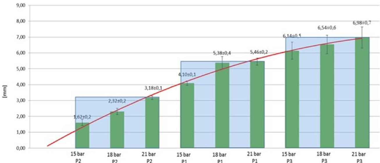
**Figure 7.** Detailed results on average coaptation increase (height of mitral leaflets coaptation) associated with small, medium, and large deformation of each P segments. The amount of deformation depends on inflation balloon pressure.
