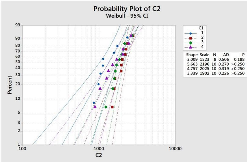
**Fig. 2** Probability plot with Weibull curves (95% CI) using maximum likelihood estimation, scale and shape values for all groups. 1: L-IDS<sup>-</sup>, 2: L-IDS<sup>+</sup>, 3: MR-IDS<sup>-</sup>, 4: MR-IDS<sup>+</sup>.
