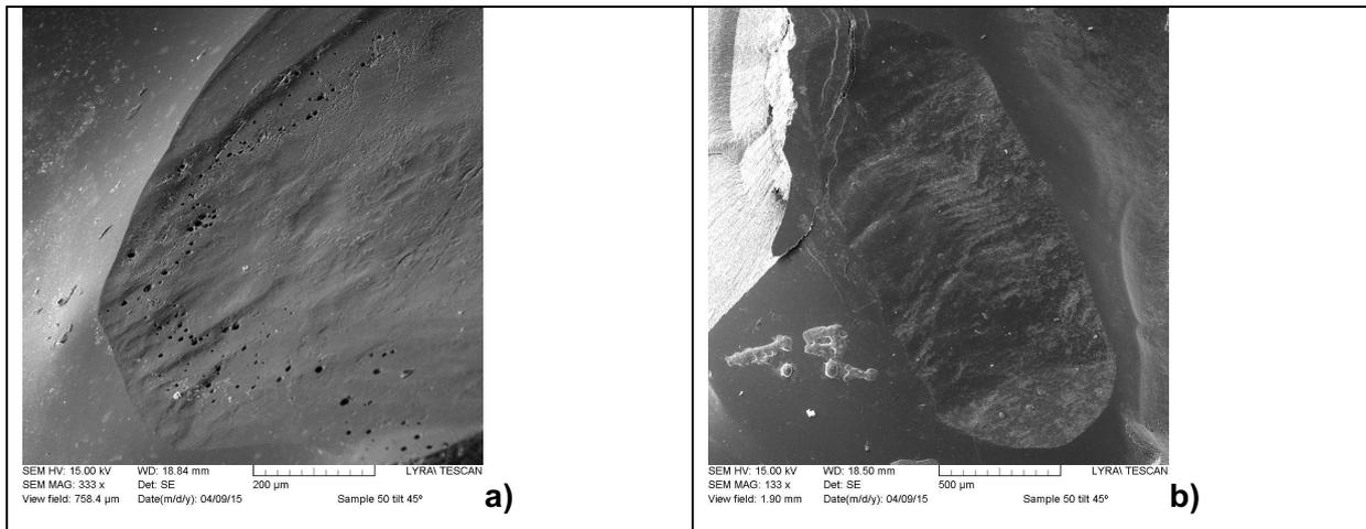
**Figs. 3a-b.** SEM images of inlays after thermo-mechanical aging from occlusal surfaces **a)** Lithium disilicate ceramic. Note the air-bubbles (\*\*) after the wear of the glaze layer (\*), **b)** Multiphase resin composite. Note the extensive wear (†) with small chippings on the occlusal surface (††).
