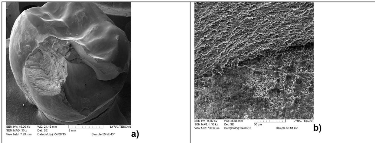
**Figs. 4a-b.** SEM images of a representative specimen from **a)** group L-IDS<sup>+</sup>. Note the fractured inlay (\*) with the IDS (Immediate Dentin Sealing) layer (\*\*) on the dentin surface (\*\*\*), **b)** group MR-IDS<sup>+</sup>. Note the interface between MR (†) and IDS (††).
