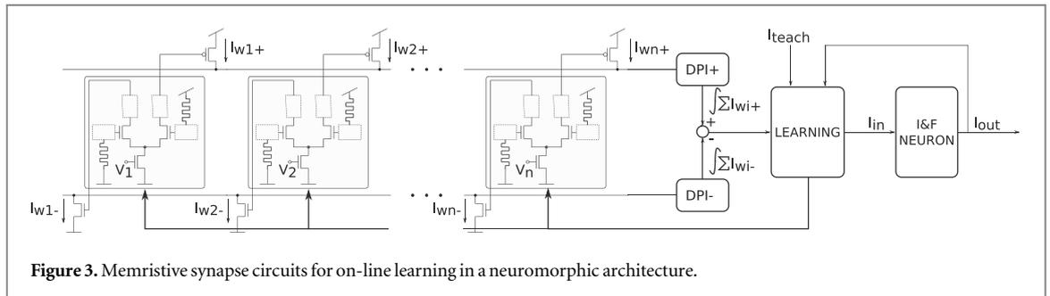
**Figure 3.** Memristive synapse circuits for on-line learning in a neuromorphic architecture.
