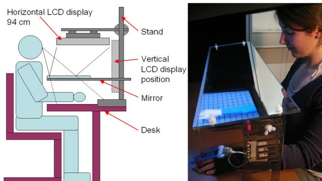
**Figure 1: Mirrored arm display. (Left) Schematic of arrangement of mirror and monitor, showing the two possible positions of the monitor. (Right) Test subject wearing data gloves and viewing screen reflected in the mirror. The arms of the subject are lying on the table below the mirror. Due to the mirror reflection, the virtual arms appear to be level with the table.**
