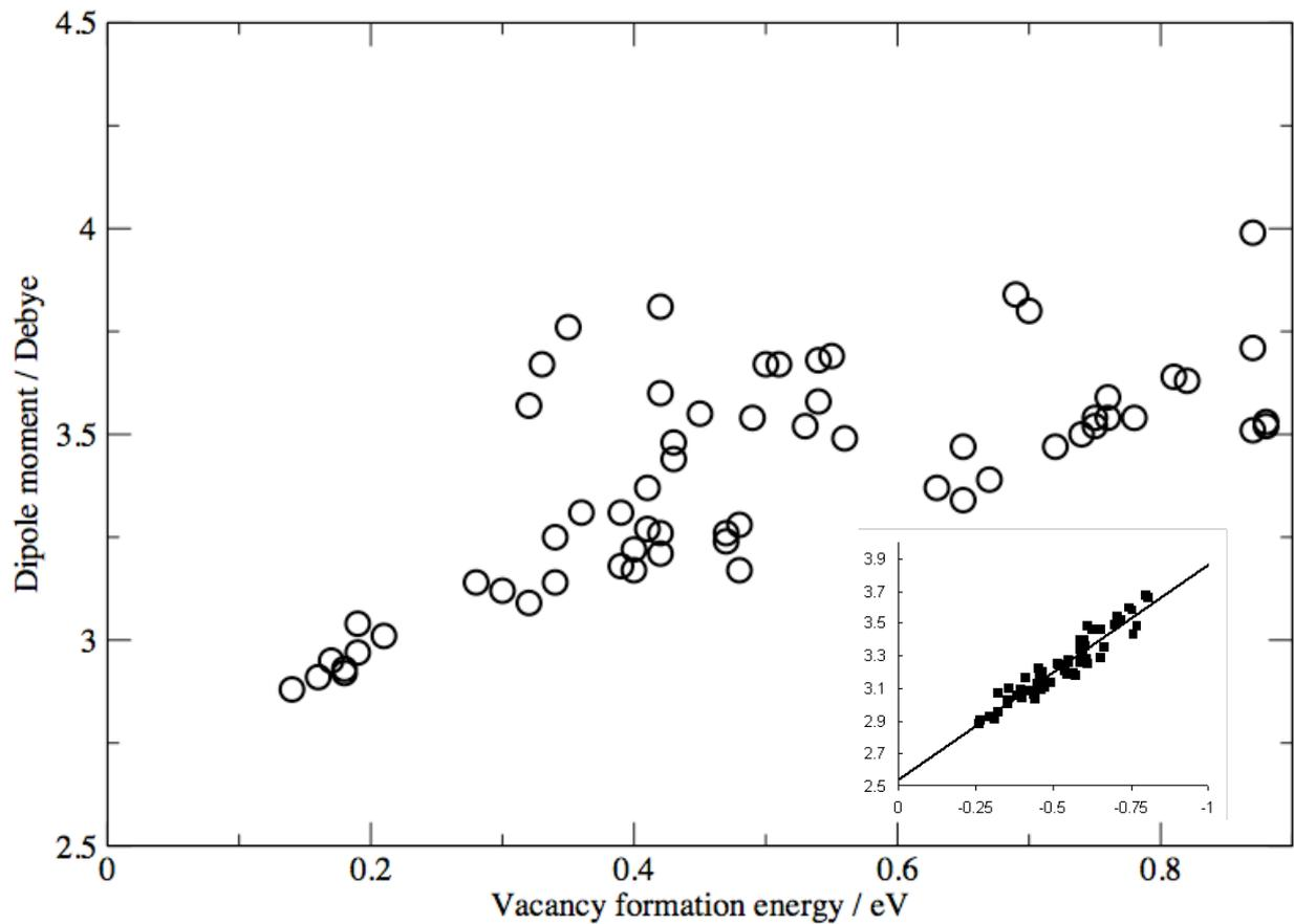
Figure 4: **Correlation between vacancy formation energy and dipole moment.** Scatter plot of the dipole moments and associated vacancy formation energies calculated for over 50 unique sites within a 6 bilayer 1h slab that exposes (0001) surfaces, showing a general positive correlation between dipole moment and vacancy formation energy. Inset into the figure is a plot of the unrelaxed defect formation energy versus dipole moment with same axis labels as the main figure.
