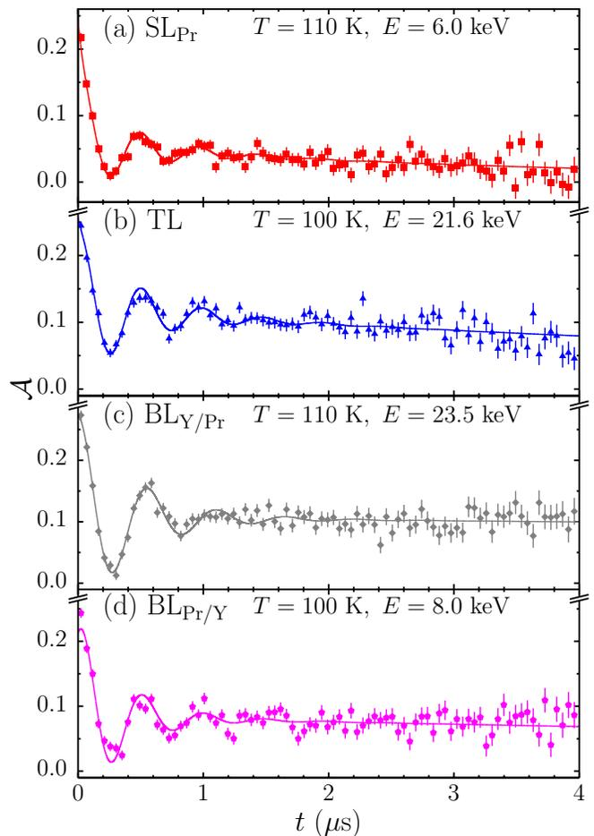
FIG. 3. (Color online) (a)–(d) Zero-field asymmetry spectra of the studied thin films listed in Tab. II at  $T = 100$  K or  $T = 110$  K, respectively. The muon implantation energies have been chosen to probe mostly the PrBa<sub>2</sub>Cu<sub>3</sub>O<sub>7- $\delta$</sub>  layers of the heterostructures. The solid lines are fits to Eq. (1).
