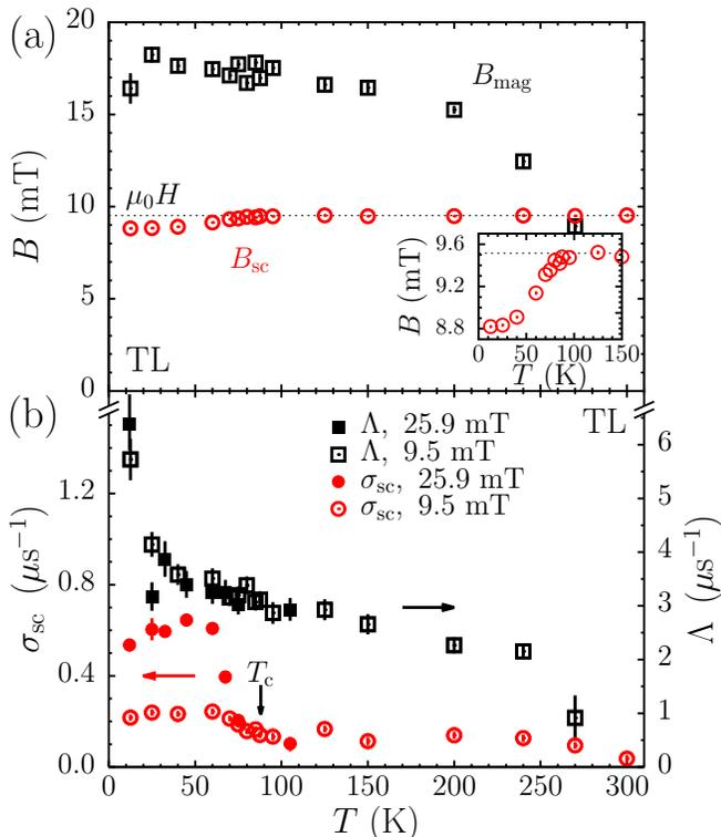
FIG. 6. (Color online) (a) Temperature dependence of the local magnetic fields  $B_{\text{sc}}$  and  $B_{\text{mag}}$  measured in an applied field of 9.5 mT probing the center of the TL structure using a muon implantation energy of 20.6 keV. (b) Depolarization rates  $\sigma_{\text{sc}}$  and  $\Lambda$  at the same energy for the highest and lowest applied fields as a function of temperature.
