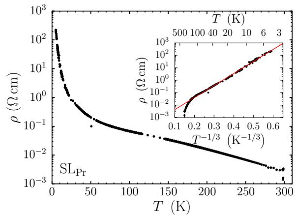
FIG. 1. (Color online) Temperature dependence of the resistivity of the SL<sub>Pr</sub> reference sample. SL<sub>Pr</sub> shows semiconducting 2D VRH behavior (measured on a film without Au capping layer). The solid red line in the inset is a fit between 5 K and 100 K using the 2D VRH formula given in the text.
