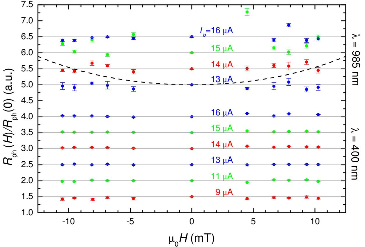
FIG. 3: Relative photon count-rates as functions of the applied magnetic field  $H$ , normalized to photon count-rates in zero-field for each  $I_b$ . For clarity, the datasets have been shifted in  $y$ -direction by multiples of 0.5. We also plotted the expected  $H$ -dependence for 985 nm photons and  $I_b = 13 \mu\text{A}$  (dashed black curve). Horizontal lines are to guide the eye.
