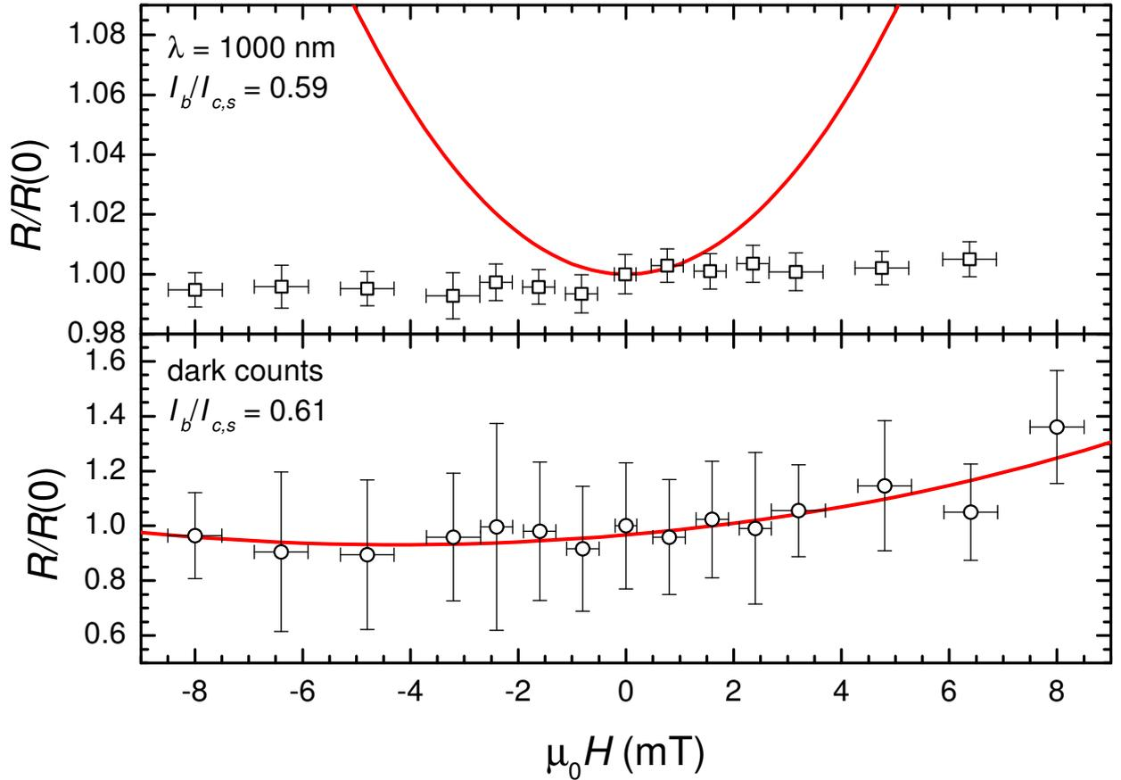
FIG. 1: Relative dark counts (lower panel) and photon count-rates (upper panel) as a function of magnetic field measured with a NbN SNSPD at  $T = 4$  K. The red line in the lower panel is a least-square fit of Eq. (4) of the main text to the data, and the red line in the upper panel is the expected field-dependence of photon count-rates according to Ref. ?. The error-bars on the x-axis stem from a preliminary-only magnetic-field calibration at the time of the measurements.
