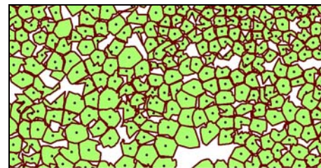
Figure 3. Detected trees and their crowns from ALS data (only a part of the study site)
