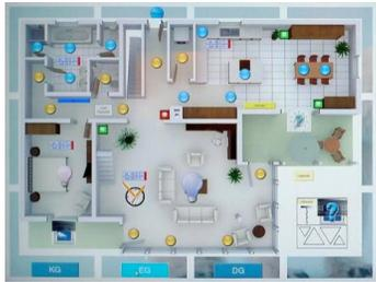
**Figure 1:** Screenshot of an example of a KNX visualization (EisBär KNX<sup>4</sup>) using floor plans
