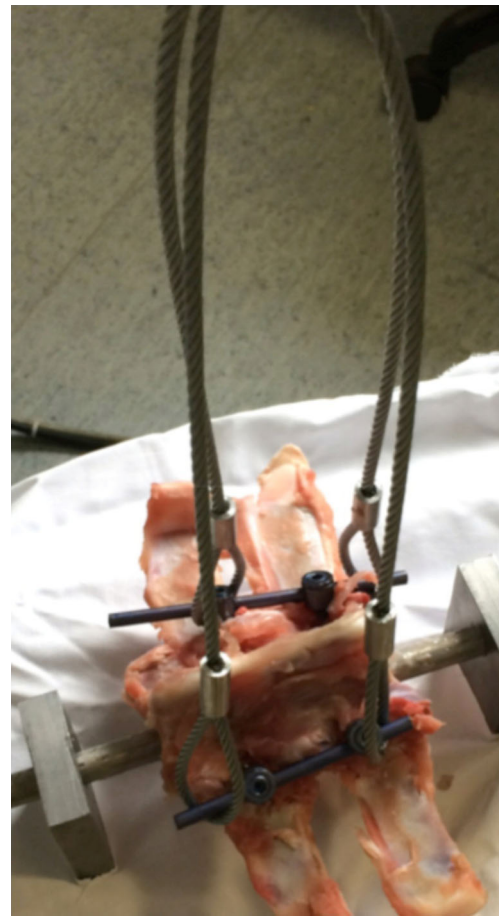
Fig. 5 Setup for biomechanical testing of pull-out strengths with a universal testing machine (Zwick-Roell, Zwick GmbH, Ulm, Germany). The segments are fixed with a steel rod (16 mm) connected to the testing machine and inserted through the spinal canal. Each end of the two rods is connected to a high-tension steel cable
