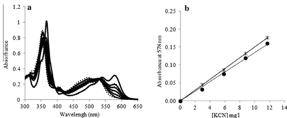
**Fig. 1.** (a) Absorbance spectra of aquacyanocobyrinic acid (33  $\mu$ M) with increasing quantity of KCN. Solid line = glycine buffer, dashed line = phosphate buffer. (b) Standard curve of absorbance read at 578 nm against concentration of KCN in linear region (2.92 to 11.7 mg/l of KCN; for details see experimental part), glycine buffer (•) and phosphate buffer (\*).
