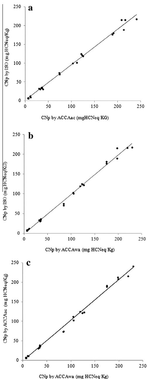
Fig. 3. Comparison of the three methods in terms of determination of total cyanogenic glycoside (CNp) by linear regression. In (a) correlation coefficient  $R^2 = 0.997$ , intercept = 1.34, slope = 0.946, standard error (SE) = 0.015. In (b)  $R^2 = 0.997$ , intercept = -0.69, slope = 1.00 SE = 0.016. In (c)  $R^2 = 0.997$ , intercept = 2.24, slope = 0.949, SE = 0.014.
