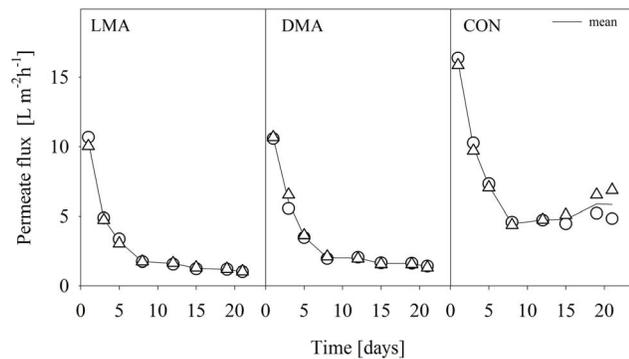
**Figure 2. Evolution of the permeate flux.** The flux is shown in  $\text{L m}^{-2} \text{ h}^{-1}$  for the filtration of differently treated feed water sources (LMA, DMA, and CON according to Figure 1). The two replicates per system are shown as circles and triangles, and are connected by the mean.
