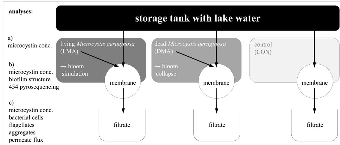
**Figure 1. Schematic view of the gravity-driven membrane (GDM) system.** Depicted are the three different operating treatments (LMA, DMA, and CON), the ultrafiltration membrane (150 kDa) and the filtrate collection. Analyses that were carried out during this study a) in the feed water, b) in/on the biofilm, and c) in the filtrate are listed on the left side of this overview.
