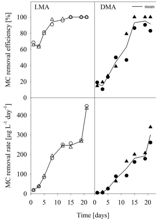
**Figure 3. Microcystin removal and removal rates.** Time course of the microcystins (MCs) removal efficiency of the GDM system (upper panel) and the MC removal rate (lower panel) in the two *Microcystis* treatments (LMA and DMA according to Figure 1). The two replicates per system are shown as circles and triangles, and are connected by the mean.
