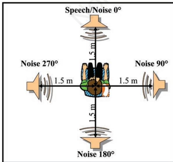
Figure 1. Test setup.
