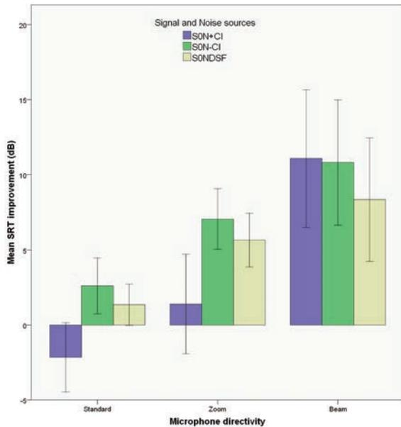
Figure 6. Improvement in speech reception threshold (SRT) for spatially separated speech and noise sources, relative to reference condition with coincident speech and noise from 0°. Mean values of  $(SRT_{S0N0} - SRT_{S0N+CI})$ ,  $(SRT_{S0N0} - SRT_{S0N-CI})$ , and  $(SRT_{S0N0} - SRT_{S0NDSF})$  and standard deviations are shown.
