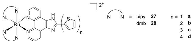
Fig. 23 Structures of Ru polypyridyl complexes conjugated with different polythiophene moieties to achieve dual Type I/II photosensitization.<sup>65</sup>
