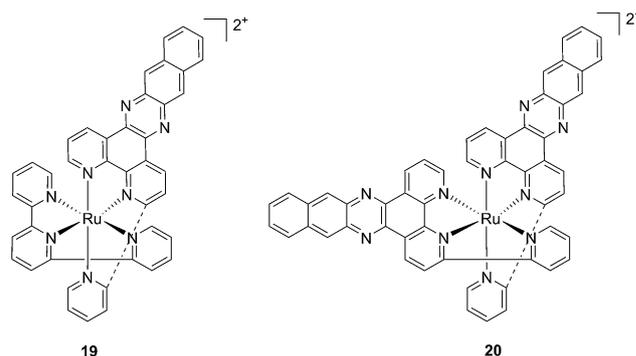
Fig. 17 Structures of the Ru complexes **19** and **20** bearing the tridentate pydppn ligand, which confers very long excited state lifetimes.<sup>57</sup>
