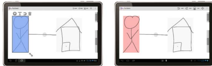
Fig. 4. A symbol on the left tablet is selected and appears in blue. On all other tablets, the symbol appears in red and is locked.
