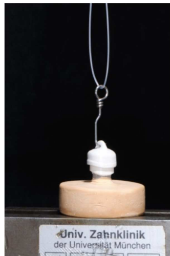
Figure 6. Experimental setup for the pull-off test: a hook pulls a zirconia secondary crown off a PEEK primary crown.
