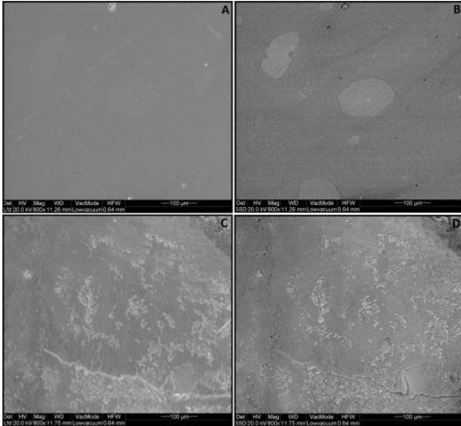
Secondary electron and backscattered electron images from the surfaces of FT-REF: A, secondary electron image; B, backscattered electron image; and FT-INV: C, secondary electron image; D, backscattered electron image (original magnification 800 times; bar = 100  $\mu\text{m}$ ).
