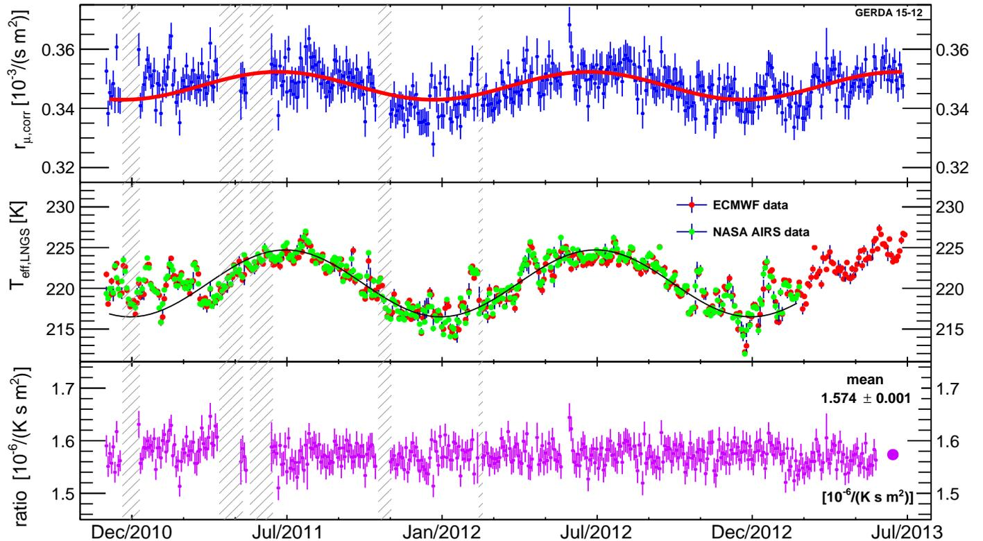
Figure 4: Top: Muon flux measured by GERDA with a binning of two days corrected for the CNGS events. A cosine with a period of 365.25 days is fit to the data. Middle: The effective temperature  $T_{\text{eff}}$  for muon production derived from data of ECWMF [13] in red and from AIRS [14] in green. The black line is a fit to the AIRS data. Bottom: the ratio of the muon rate and the  $T_{\text{eff}}$  from the ECWMF data set is shown to be flat over the entire time.
