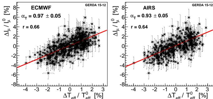
Figure 5: Dependence of the change in muon rate on the change in effective temperature, for both sets of temperature data. A linear fit ( $\chi^2/\text{ndf}_{\text{ECWMF}}=391/410$ ,  $\chi^2/\text{ndf}_{\text{AIRS}}=364/351$ ) yields values for  $\alpha_T$ .
