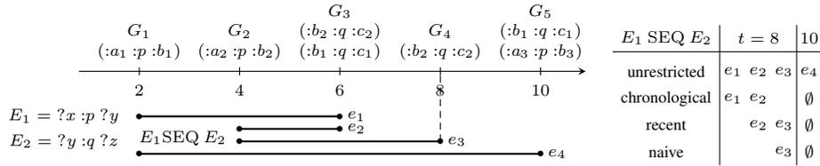
Fig. 1: Illustration of the running example. The stream, on the top left, composes of five items  $(G_1, 2) \dots (G_5, 10)$ . Events matched the pattern  $E_1$  SEQ  $E_2$  are depicted below the timeline. The bold lines denote the intervals that justify the events. The table on the right shows the results produced with regards to different policies.
