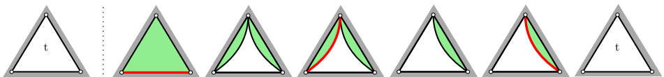
FIG. 7. The three peeling steps needed to peel a simple triangle (on the left). The external face is in gray, the unexplored regions are in green and the edge to peel at each step is in red.
