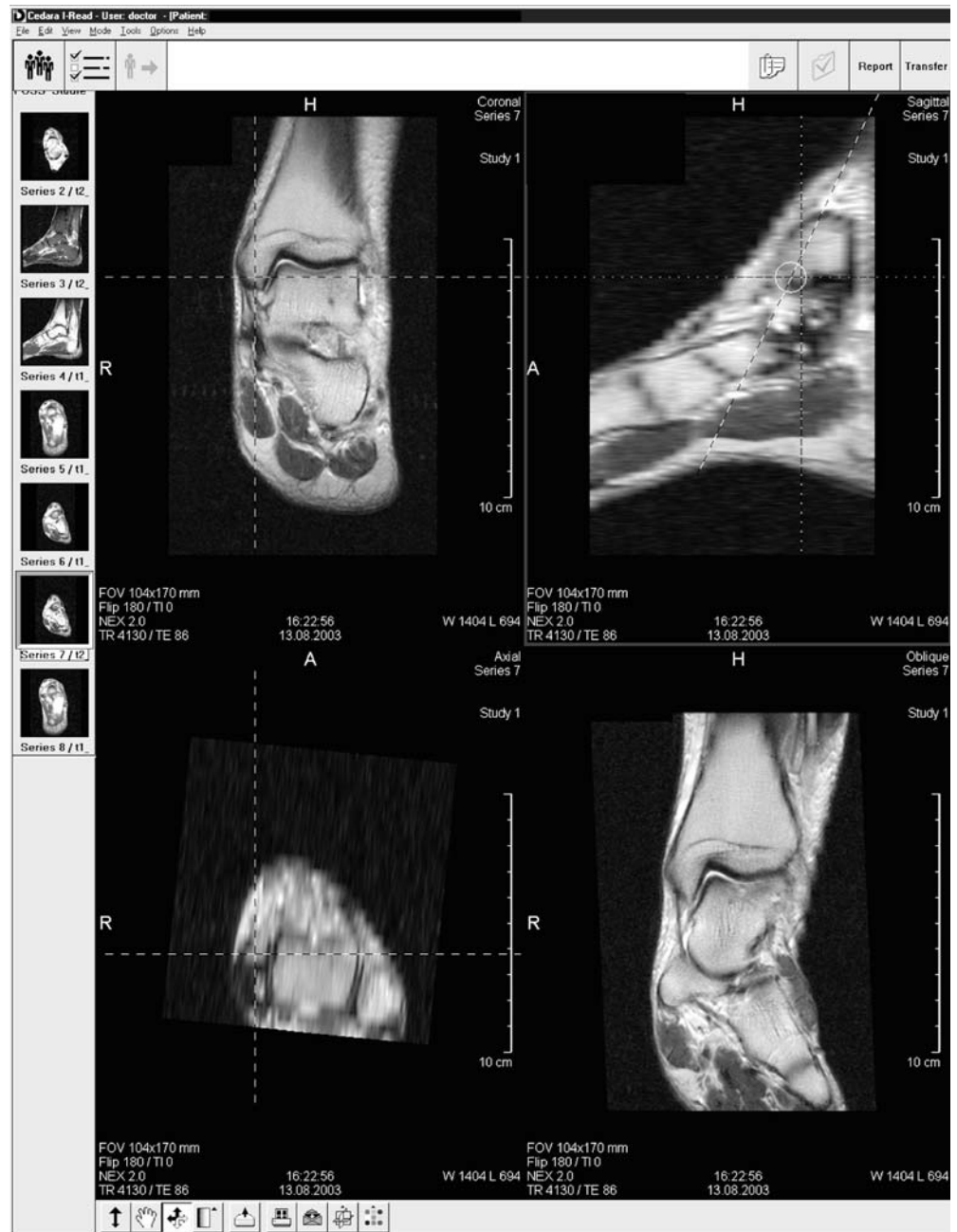
Fig. 1 Screenshot of MPR tool. Source image is shown on the upper left quadrant. The automatically provided planning planes are shown on the upper right and lower left quadrants. Note oblique reformation plane (dashed white and black line) on the upper right quadrant. The resulting MPR appears in the lower right quadrant
