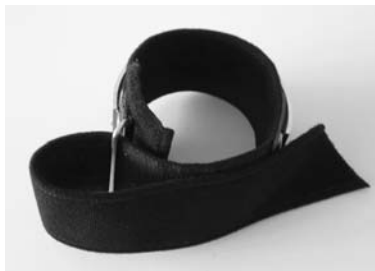
Fig. 3 Cuff that connects the rotary module with the human upper arm
