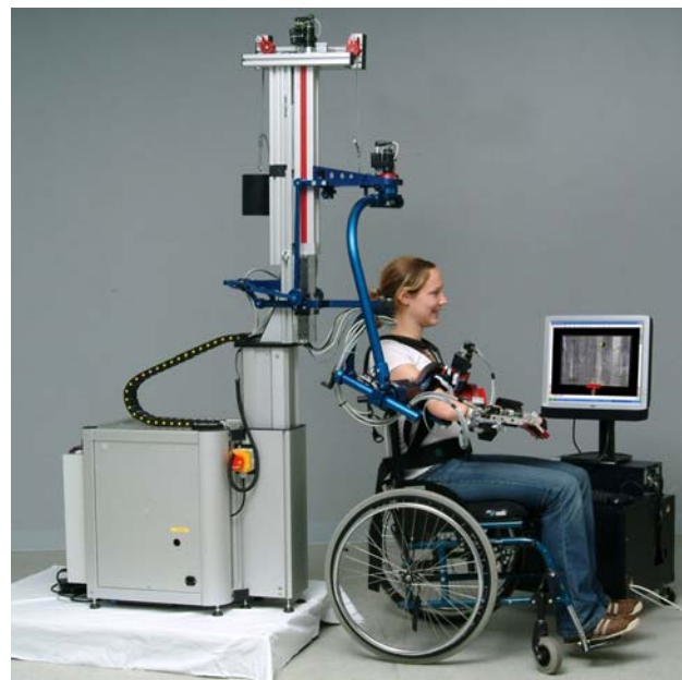
Fig. 12 ARMin II—New version with 6DOF and statically determined shoulder actuation
