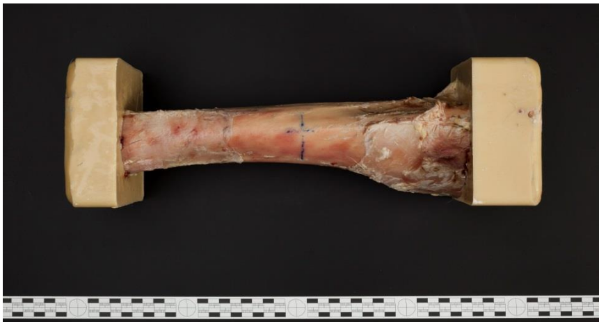
Fig. 1: Dissected left tibia with the proximal and distal ends embedded in polyurethane. The blue cross indicates where the impactor was intended to impact the bone.
