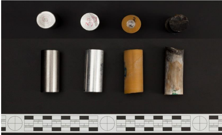
Fig. 3: Impactor heads: cylindrical steel, aluminium, polyurethane and hoof horn bars (from left to right).
