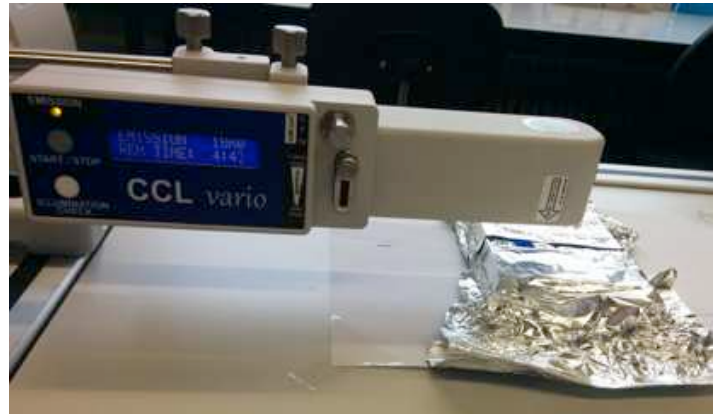
Figure 3: UV-A irradiation with CXL-lamp.
