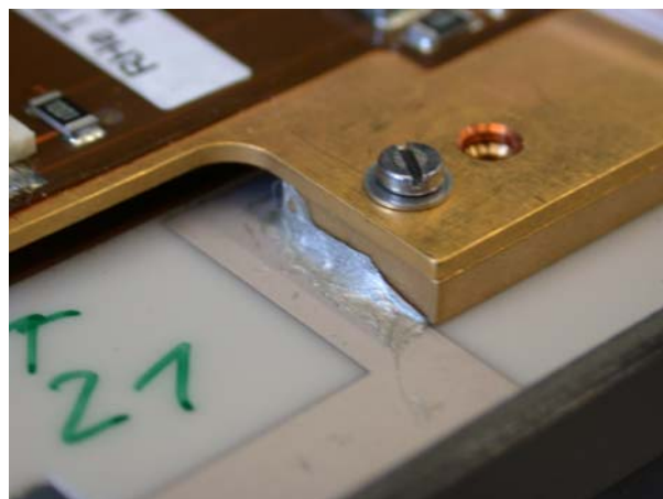
Figure 2: Breakup of silver glue after thermal cycling
