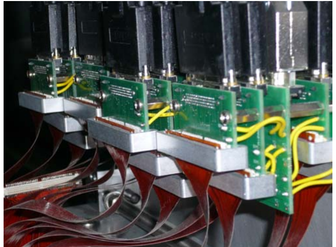
Figure 4: machined aluminium clamps for securing the high-density connectors
