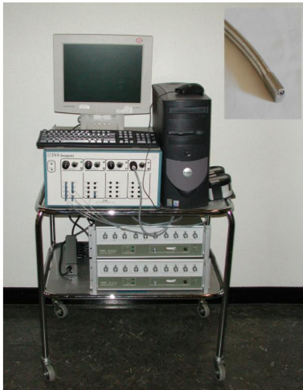
Fig. 1. The FD-NIRS instrument used for the present study is shown. The inlet shows the cervical probe specially manufactured for this study. [Figure can be viewed in color online via [www.interscience.wiley.com](http://www.interscience.wiley.com).]
