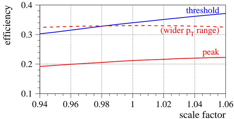
**Figure 9:** Variation of the selection efficiencies ( $\epsilon_{\text{th}}$  and  $\epsilon_{\text{pk}}$ ) with an overall energy scale factor. The two solid lines show the variation obtained with our nominal cuts, at  $\sqrt{s_{\text{th}}}$  and  $\sqrt{s_{\text{pk}}}$ . The dashed line shows what we would obtain if we applied a looser  $p_T$  cut at  $\sqrt{s_{\text{pk}}}$ .
