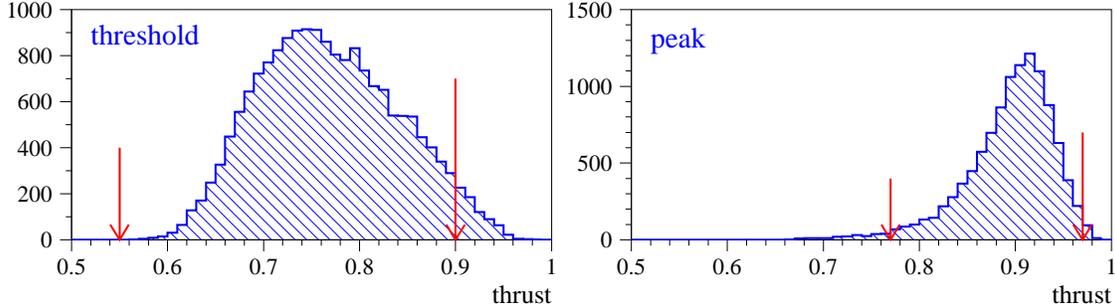
**Figure 4:** Signal marginal distributions for the thrust, at  $\sqrt{s_{\text{th}}}$  (left) and at  $\sqrt{s_{\text{pk}}}$  (right). The arrows indicate the cuts chosen to minimize the systematic uncertainties as well as the statistical uncertainty.
