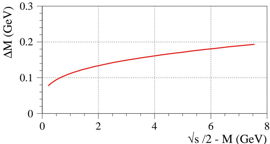
**Figure 1:** Statistical uncertainty on the mass,  $\Delta M_X$ , as a function of the beam energy above threshold,  $\sqrt{s}/2 - M_X$ . This result is based on a Feldman-Cousins confidence belt construction, with a simple Ansatz for  $\sigma(M_X)$  and approximate values for  $\epsilon$  and  $\mathcal{L}$ . Backgrounds were not taken into account.
