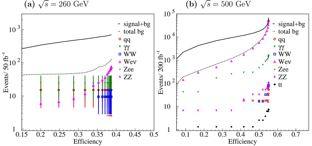
**Figure 8:** Performance of the Iterative Discriminant Analysis (IDA) for  $\sqrt{s} = 260$  GeV and  $\sqrt{s} = 500$  GeV. The plots show the remaining background event numbers for unpolarized beams as a function of the signal efficiency.
