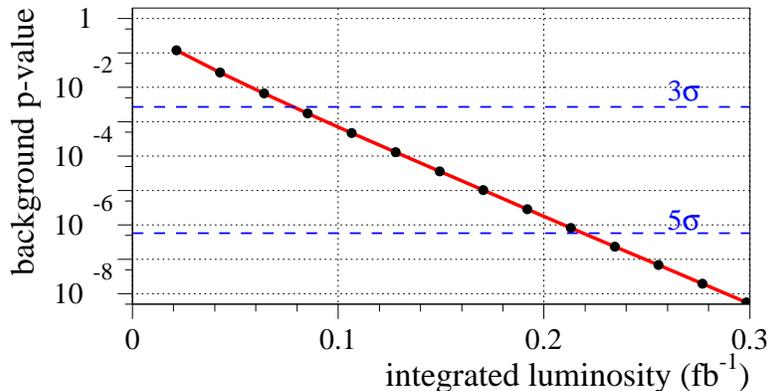
**Figure 14:**  $p$ -values as a function of integrated luminosity  $\mathcal{L}$ . The black dots on the line show hypothetical integral numbers of observed events, starting at  $N = 1$  for  $\mathcal{L} = 0.02 \text{ fb}^{-1}$ .
