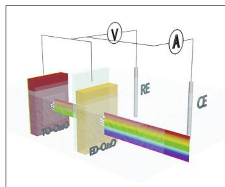
Fig. 6. Schematic diagram of the dual  $\text{Cu}_2\text{O}$  photocathode experiment. The transparent electrodeposited (ED- $\text{Cu}_2\text{O}$ ) photocathode is placed in front of the thermally oxidized (TO- $\text{Cu}_2\text{O}$ ) photocathode, enabling efficient photon conversion over the entire absorption spectrum. Reproduced from ref. [15] with permission from Wiley.
