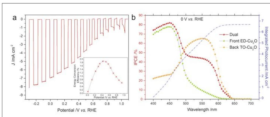
Fig 7. a) The PEC and b) IPCE of the dual Cu<sub>2</sub>O photocathode. Inset of a) is the thermodynamical-based energy conversion efficiency. Reproduced from ref. [15] with permission from Wiley.
