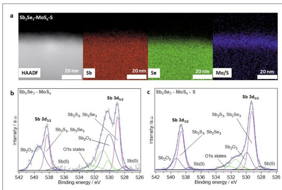
Fig. 2. a) STEM HAADF image and EDX elemental mapping of Sb<sub>2</sub>Se<sub>3</sub>-MoS<sub>x</sub>-S (sulfurized). b) XPS core level spectrum of Sb 3d for Sb<sub>2</sub>Se<sub>3</sub>-MoS<sub>x</sub> (non-sulfurized). c) XPS core level spectrum of Sb 3d for Sb<sub>2</sub>Se<sub>3</sub>-MoS<sub>x</sub>-S (sulfurized). Reproduced from *J. Mater. Chem. A* **2017**, *5*, 23139 with permission of the Royal Society of Chemistry.
