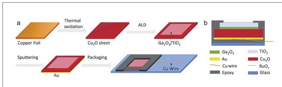
Fig. 5. a) Procedure for fabrication of the TO- $\text{Cu}_2\text{O}$  photocathode. b) Cross-section view of the photocathode (not to scale). Reproduced from ref. [15] with permission from Wiley.
