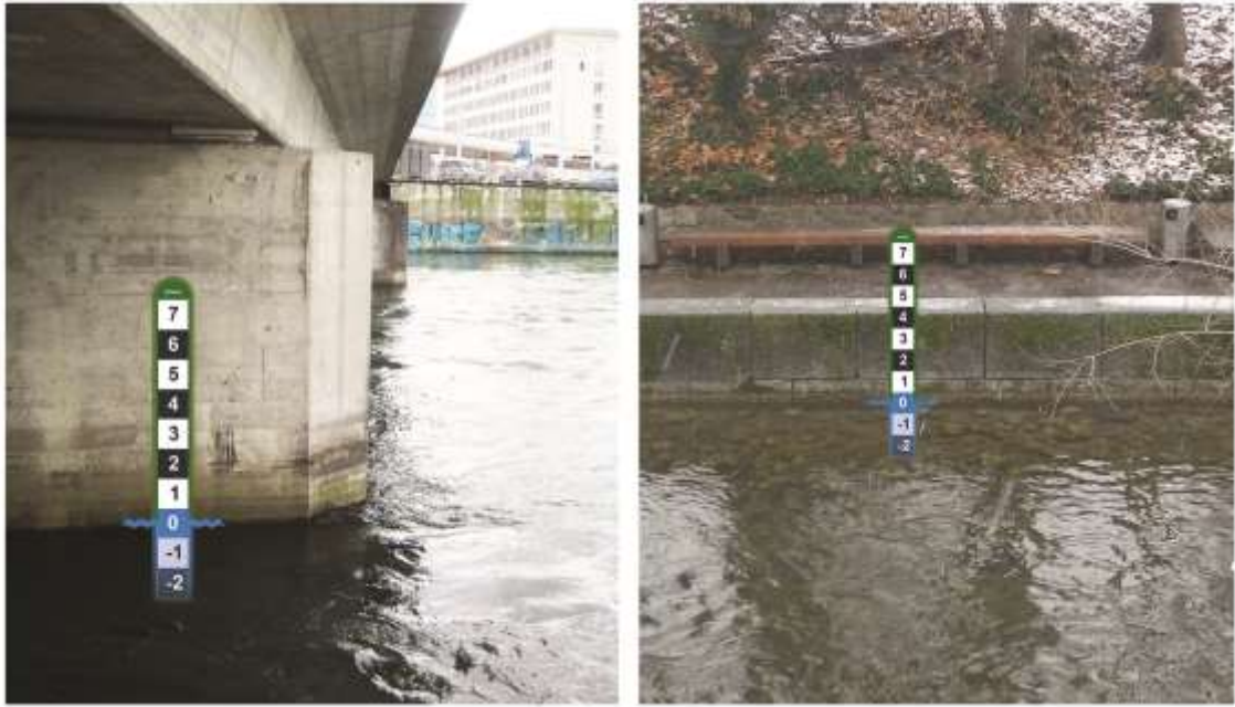
Figure 1. Example of a virtual staff gauge in the pictures used for the field survey at Limmat (left) and Schanzengraben (right). Photographs taken on 29.06.2016 when the streamflow was 165\text{m}^3/\text{s} (Limmat) and on 05.01.2017 (unknown streamflow; Schanzengraben). For the dates and the flow conditions during the surveys see Table 1.
