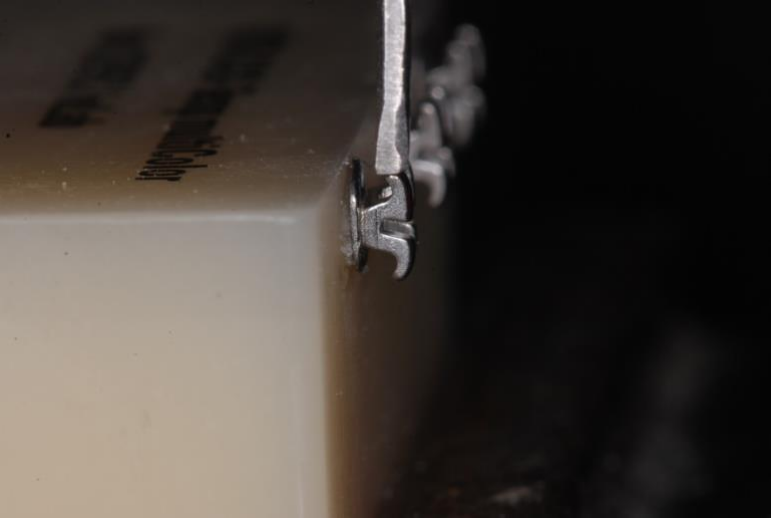
Fig. 1. The experimental set-up for bracket shear bond strength testing
