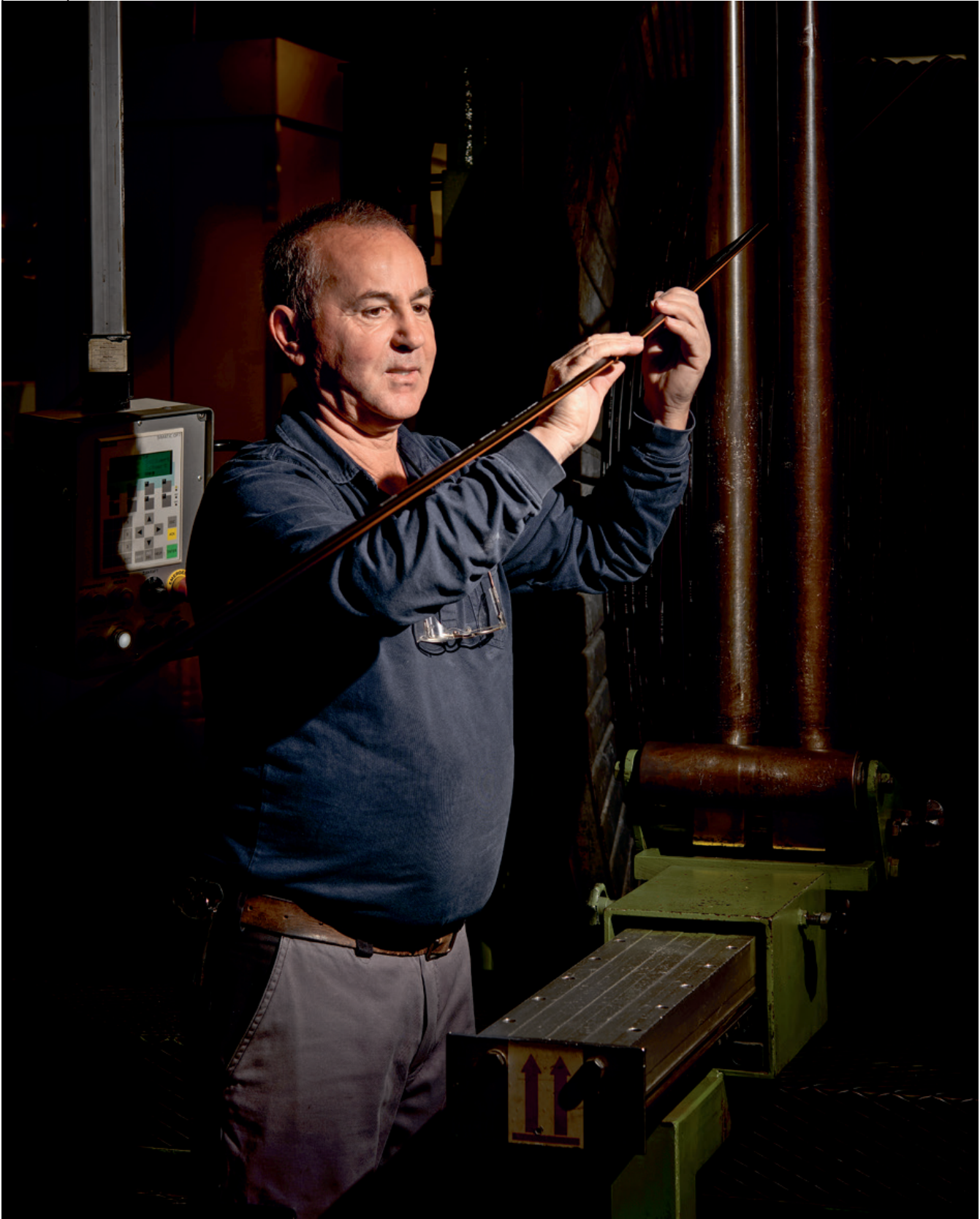
Visual check of the completed cable.
