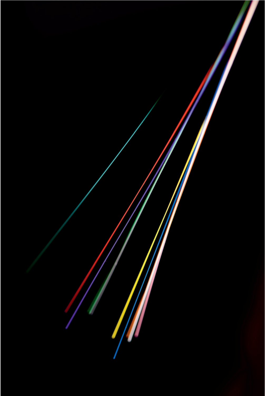
Color-coded optical fiber strands.
