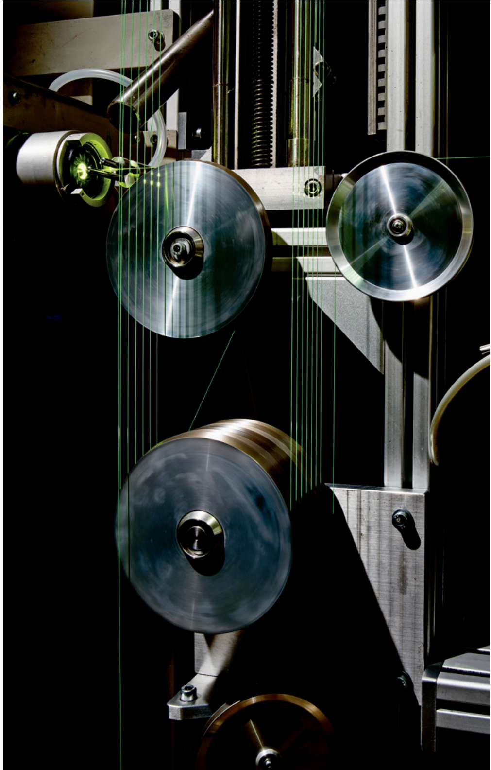
Fiber strands come color-coded in twelve basic colors, here green.
