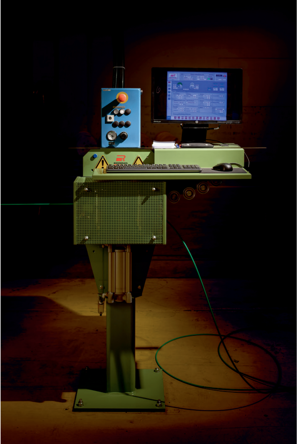
Quality check: The cable is measured and labeled.
