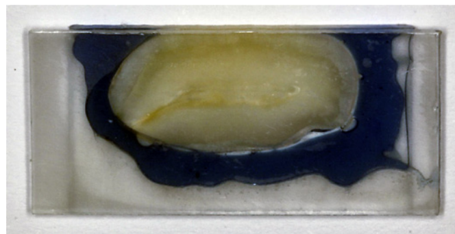
Fig. 2. Enamel sample placed between two polycarbonate platelets and embedded in a light-curing resin.
