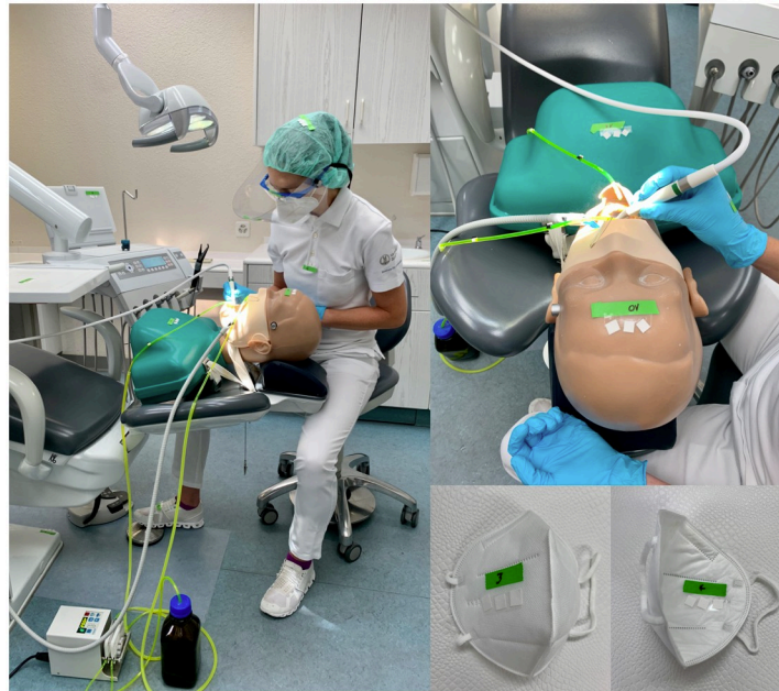
Fig 1. Depiction of the experimental set-up, the dental unit and the exemplified demonstration of adsorbent filters and their fixation via double-sided adhesive tapes.
