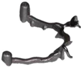
Figure 6. Lateral view of additively manufactured cobalt-chromium alloy framework.
