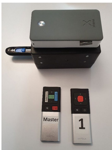
Figure 6. Recording device containing the sensor, the battery (gray) and an USB stick for data storage; remote for the experimenter (Master); remote control for subject (1).
