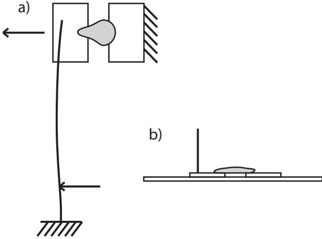
**Figure 1.** Schematic of the mechanical forcing setup. A top view is shown in a), while a side view is shown in b). The wing disc (grey) is attached to two glass cover slides, one of which is attached to a surface. The other cover slide is fixed to a spring sheet, which is forced by a translation stage at a given distance. This gives a controllable force ranging from  $1\mu\text{N}$  to several mN, which is ideally suited to study epithelial tissues.
