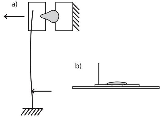
**Fig. 1.** Schematic of the mechanical forcing setup. A top view is shown in a), while a side view is shown in b). The wing disc (grey) is attached to two glass cover slides, one of which is attached to a surface. The other cover slide is fixed to a spring sheet, which is forced by a translation stage at a given distance. This gives a controllable force ranging from  $1 \mu\text{N}$  to several  $\text{mN}$ , which is ideally suited to study epithelial tissues.
