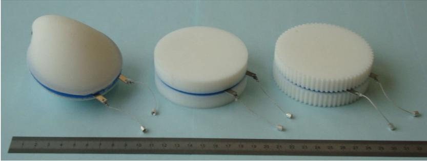
Figure 3: Plastic shells with a peripheral rubber tube (blue) with holes to emit water. The two strings with screw couplings allow easy attachment and detachment of the shell. The picture shows the three shells compared in the results section (from left): smooth bivalve shape, smooth disk shape and ridged disk shape.
